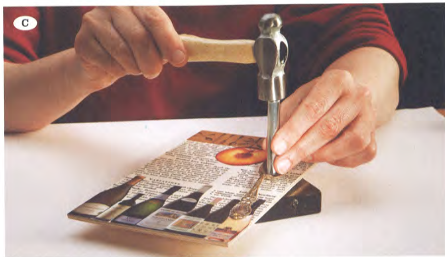
Use a hammer and rivet setter to set the cap in place.
